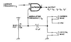
fig. 3. Using the SN7400 gate as a product modulator (mixer).
